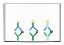
Biotinylated detection antibodies specific for the target are added to bind another epitope on the target antigen.
