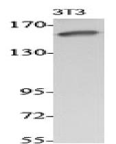
Western Blot analysis of various cells using ASK 1 Polyclonal Antibody diluted at 1:1000
