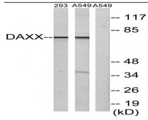
Western blot analysis of lysates from 293 cells and A549 cells, using DAXX Antibody. The lane on the right is blocked with the synthesized peptide.
